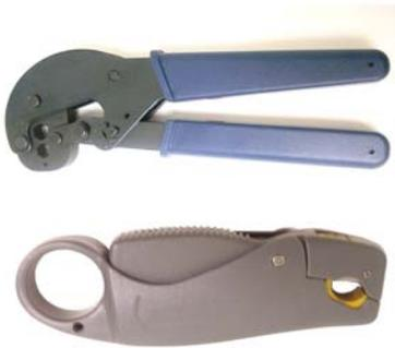
*Crimp Tool and Strip Tool for TWS-400 Cable Displayed*
