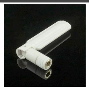
Ventev's Tri-Band ABS Antenna is designed to operate with any manufacturer's access point that utilizes RPSMA connectors. This antenna operates in the 2400-2500 and 5150-7125 MHz frequency range with a gain of 3/4/3.5 dBi across the band. The antenna includes a direct RPSMA Male connector and is designed to support demanding wireless applications.
