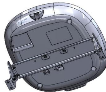
**Aruba 300 series APs and older** come with a factory T-bar clip. Attach the supplied T-bar to AP adapter bracket with supplied qty 2 #6-32 screws. Attach AP adapter bracket with T-bar to the wedge bracket using 2 screws inserted from under wedge bracket. Snap AP to T bar.
