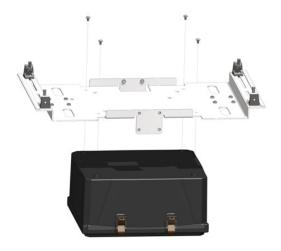
5) Bracket assembly can be installed vertical or horizontal. Slide I beam clamps to engage I beam and hand tighten I-beam bolts. Once bracket is centered, tighten I beam bolts with a wrench.
