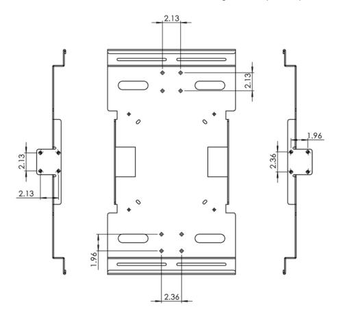
All holes have  $\frac{1}{4}$ -20 inserts. 1.96 x 2.36 hole pattern is for the omni antenna brackets. The 2.13 x 2.13 hole pattern fits the TerraWave Universal Articulating Mount, the optional TerraWave Industrial Articulating Mount and the optional Patch Antenna Paddle.
