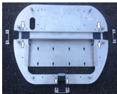
Railing Brackets Removed
