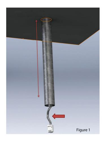
Step 3 - Attach the hanging conduit mount to the conduit with a conduit nut (not supplied). Shown in Figure 2.
