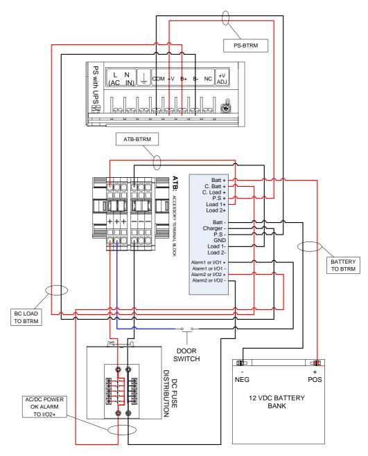
Figure 1: UPS Enclosure System with BTRM.
