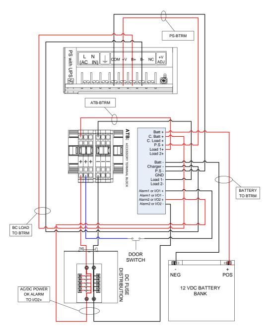
Figure 3: Power Supply with UPS Enclosure System with BTRM.
