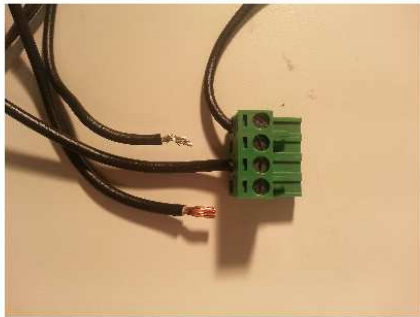
REMOVE THERMAL SWITCH WIRES FROM POE MODULE TERMINAL BLOCK
