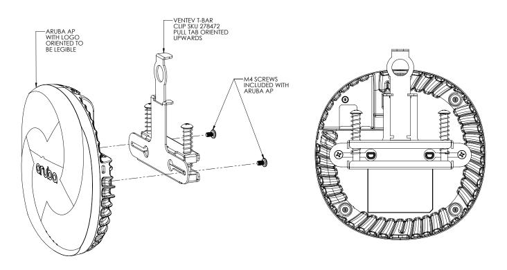
First, remove any factory brackets from the access point prior to Ventev Aruba T-Bar Clip installation. Retain the two (2) M4 screws used to hold the factory bracket in place.
